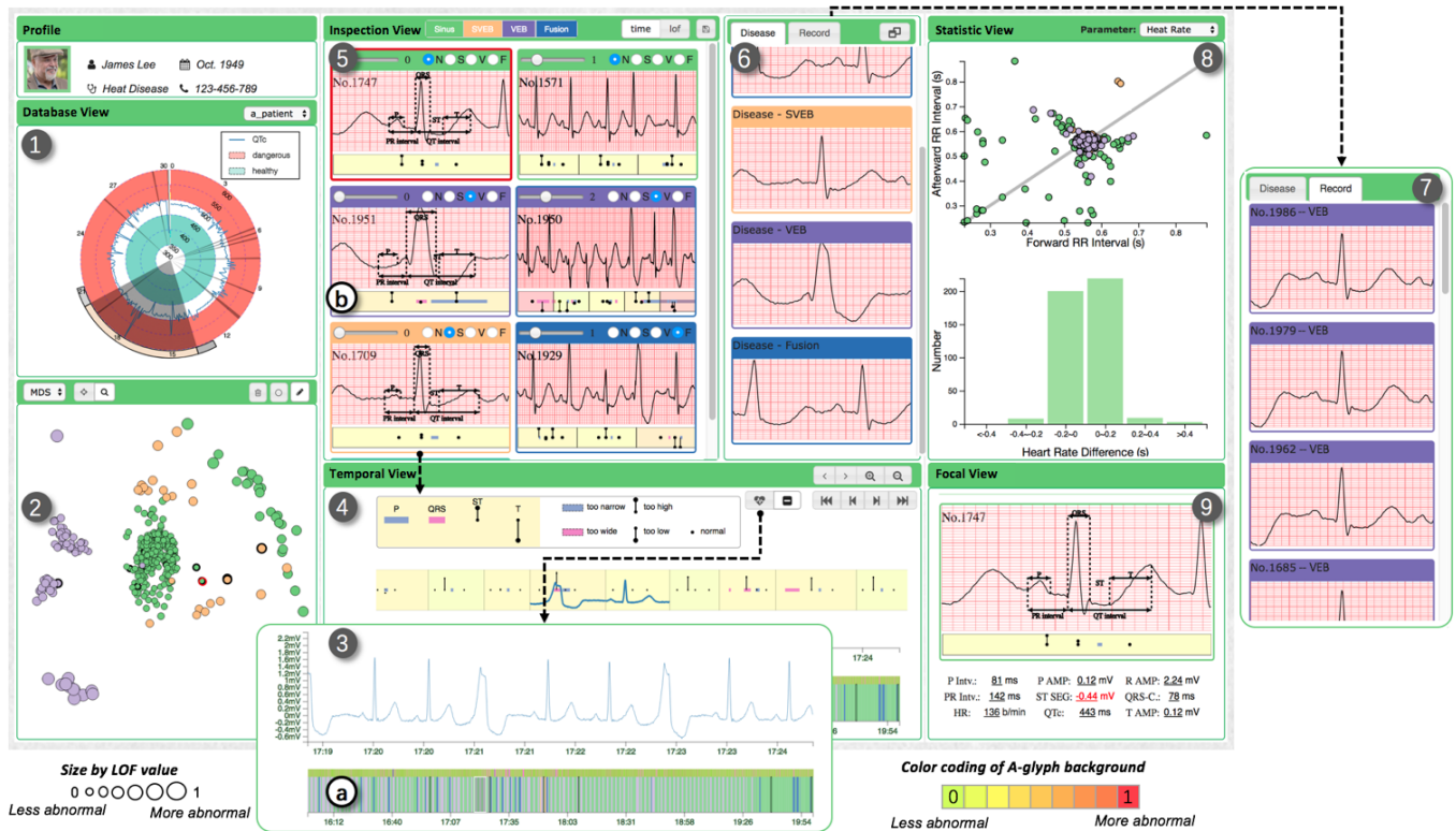
Figure 2. The ECGLens system contains nine interactively coordinated views, including (1) a view illustrating the entire series of raw ECG waves in a circular timeline, (2) a view showing the distribution of heartbeats in a feature space, (3) conventional & (4) glyph representations of a segment of the ECG waves selected from view (1), (5) an inspection view depicting the details of the selected heartbeats, (6) a cluster view showing a list of clustered anomalous heartbeats with the details of each cluster shown in (7), (8) a view showing the statistics of the heartbeats under investigation, and (9) a focal view showing the details of one single selected heartbeat.
