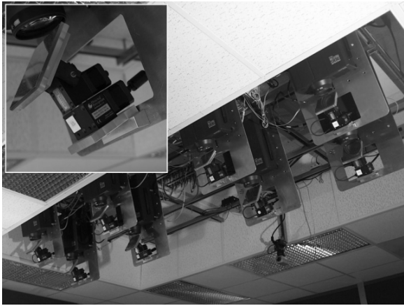
Figure 3: The PixelFlex projector array.
